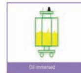
Oil immersed Hermetically sealed transformer for more compact dimensions of the substation, with oil retention tank.
